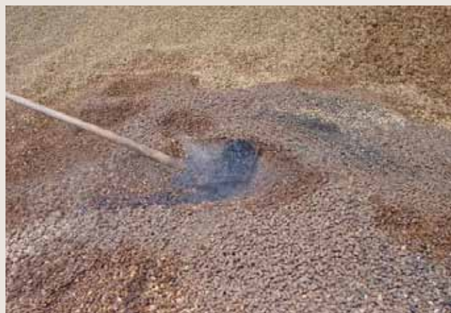
^ Smoking seedcake cargo. Double bottom fuel oil heating should be managed
