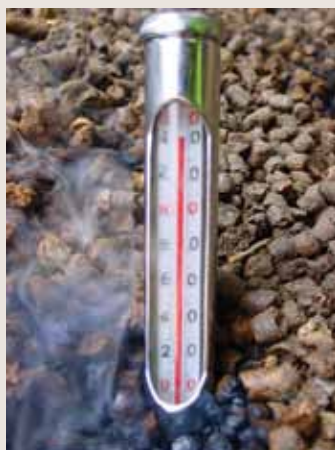
^ Have a thermometer onboard in order to take cargo temperature
