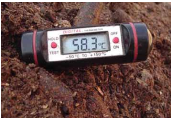
^ Temperature reading taken during self-heating leading to spontaneous combustion
