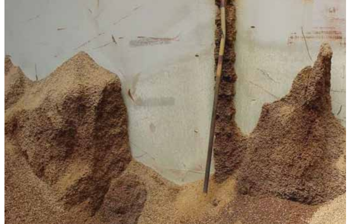
^ Seedcake damage showing a broken temperature gauge
