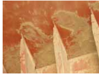
^ Cement residues in less accessible parts of the hold
