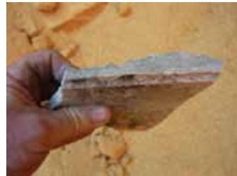
^ Large pieces of cement contaminating the cargo
