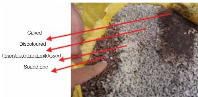
^ Condition of wetted cargo in comparison with sound one
