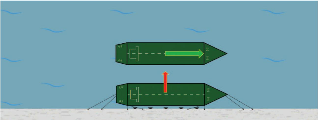
D. As the passing vessel starts to draw clear, the moored vessel will normally surge in the direction of travel of the passing vessel, will sway towards the berth and the end of the vessel closest to the passing vessel will yaw away from the berth.
