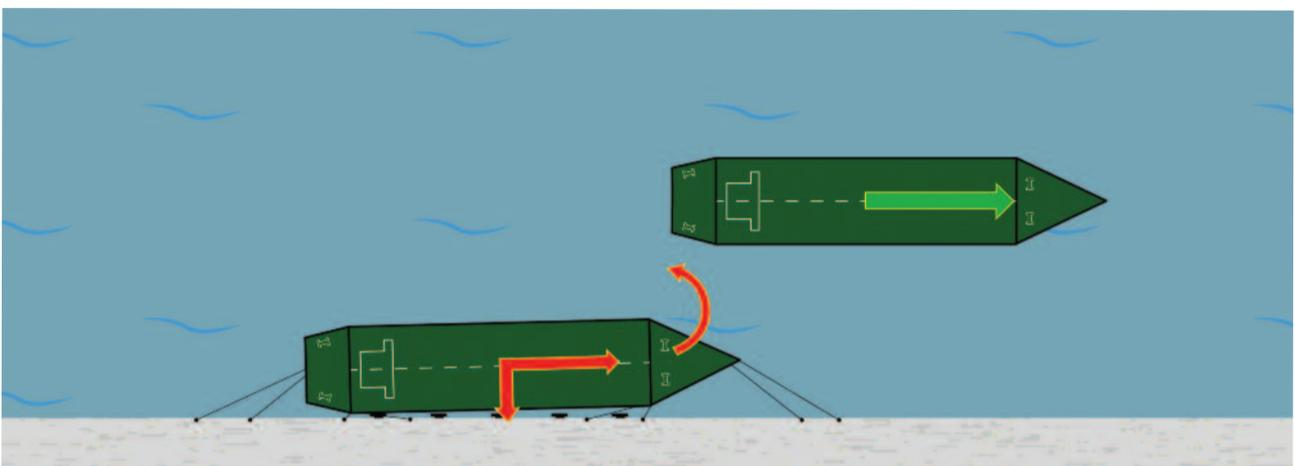
The magnitude of the hydrodynamic forces imparted in a moored vessel, causing it to surge, sway and yaw at its berth, will depend on a complex array of factors, including, but not limited to the following:
